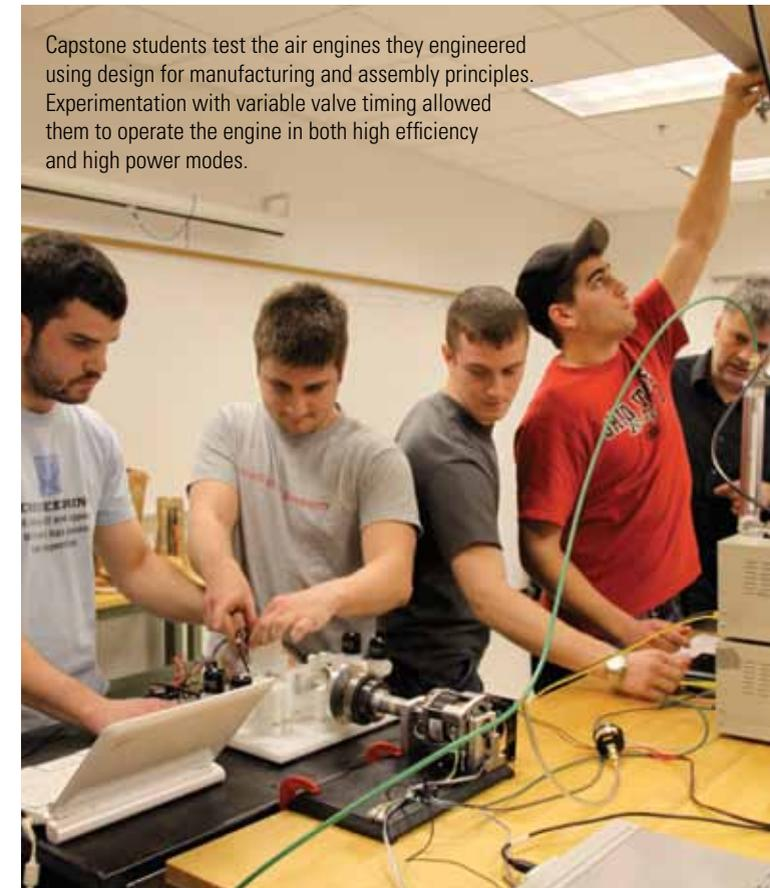
Capstone students test the air engines they engineered using design for manufacturing and assembly principles. Experimentation with variable valve timing allowed them to operate the engine in both high efficiency and high power modes.
